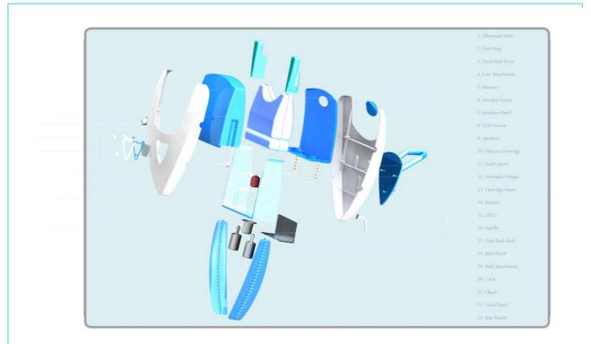
Identification of features, which facilitate assembly/disassembly for recycling
